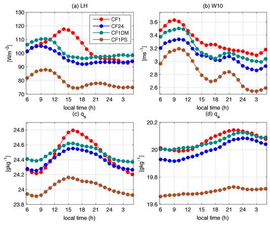
FIG. 5. The hourly composites of (a) latent heat flux (W m<sup>-2</sup>), (b) 10-m wind speed (m s<sup>-1</sup>), (c) saturation specific humidity at the temperature of the ocean surface (g kg<sup>-1</sup>), and (d) the specific humidity of air at 2 m (g kg<sup>-1</sup>) during the suppressed phase of MJO2.
