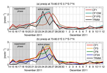
FIG. 8. Time series of daily-mean total precipitation rates (mm h<sup>-1</sup>) over the NSA region (0.7°S–7°N, 73°–80.5°E) of (a) CF1, CF1DM, CF1PS, and TRMM, and (b) CF1, CF3, CF6, CF24, and TRMM. The gray boxes delineate the periods of the convectively suppressed (15–19 Nov 2011) and active (20–26 Nov 2011) phases of MJO2.
